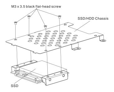
Figure 4-14 Removing the SSD/HDD chassis
